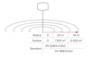
How to read the drawing: in a range of 44 m, being a surface of 6000  $\ensuremath{\text{m}}^2$ , we guarantee a lighting in accordance with the EN1838 standard.
